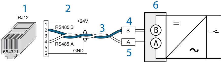
Figure 4: Connecting the inverter
