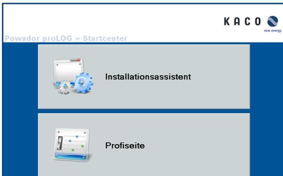
The Installation Wizard has been designed to make it as easy as possible for the user to set up the data logger. The installation procedure comprises 14 steps. Help is provided for each step.
