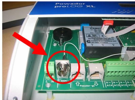
The antenna connection is located in the connection area, next to the 230 V grid connection. Connect the included antenna here.
