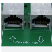
You can connect up to 100 current sensors (Powador-go) to the "Powador-go" RJ45 sockets. For example, you can use the current sensors to include inverters without RS485 in monitoring.
