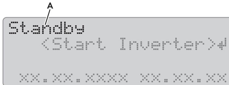
Figure 4: Display of operating states (example: Standby)
