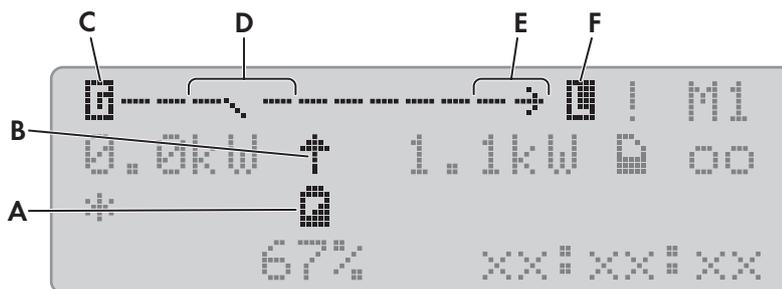
Figure 7: Energy flow diagram in standard mode (example)
