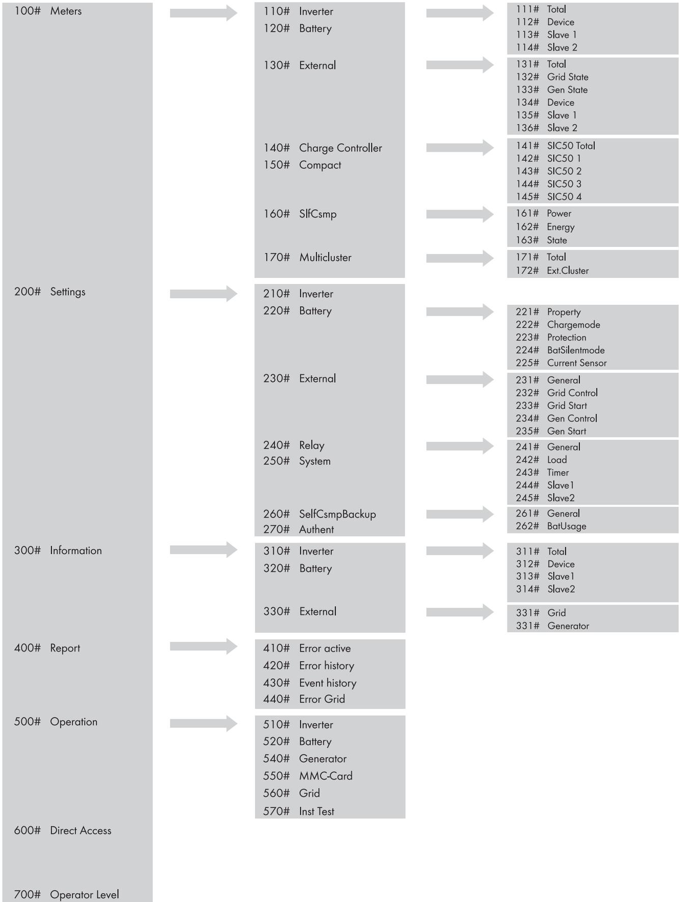
Figure 20: Menu structure: installer mode and expert mode
