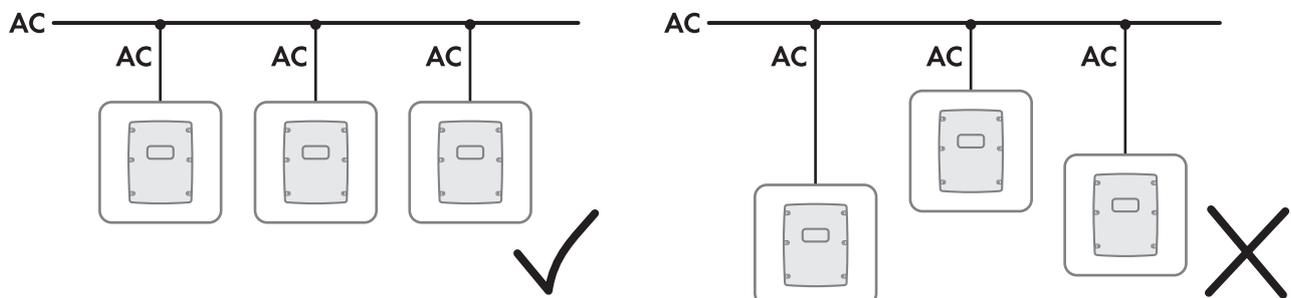
Figure 10: Correct, symmetric connection and incorrect, asymmetric connection of the Sunny Island inverters
