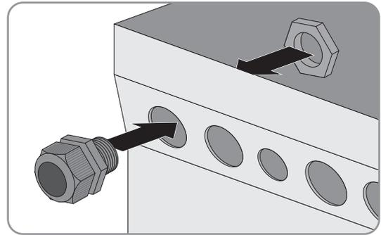
3. When connecting the cable to connection **AC2**, attach the M25 cable gland to the **AC2** enclosure opening using the counter nut (torque: 7 Nm).
