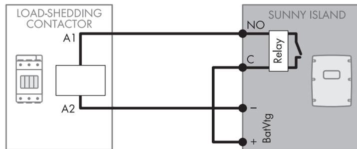
Figure 17: Connection of control cable for one-level load shedding (example)
