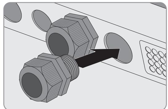
6. Lead the **DC+** cable through the **DC+** cable gland into the Sunny Island.
