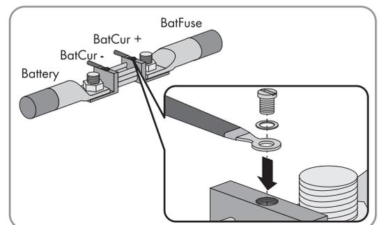
3. Connect the **BatCur-** insulated measuring conductor to the side for connecting the battery on the battery current sensor.
