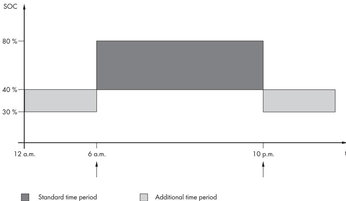
Figure 26: Profile of the SOC and the times for generator requests
