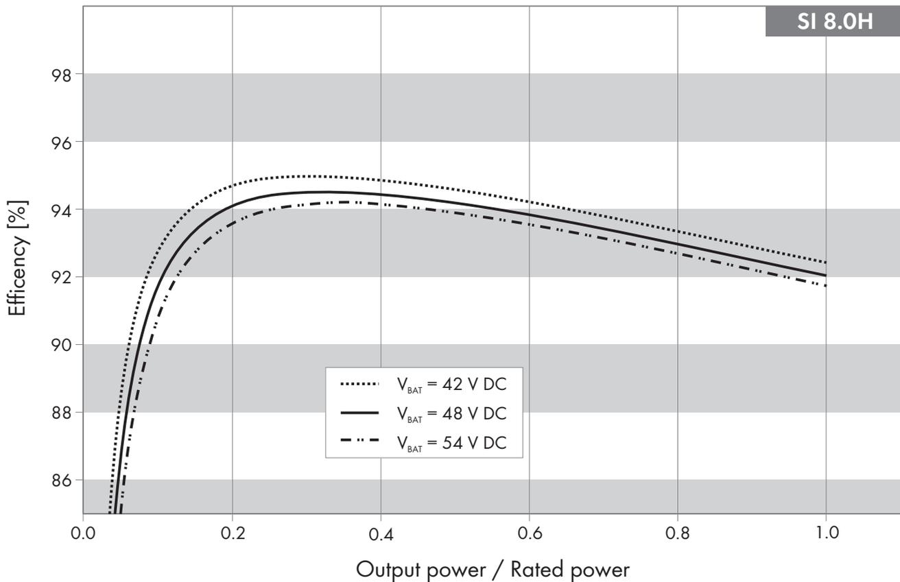
Figure 31: Characteristic efficiency curve
