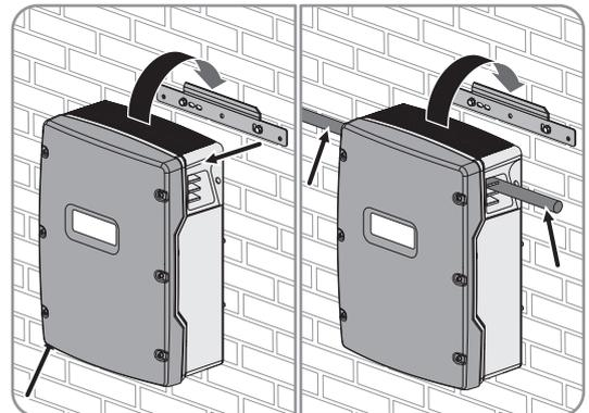
8. Use an Allen key (AF 5) to attach the Sunny Island to the wall mounting bracket on both sides with the M6x10 screws provided (torque: 4 Nm to 5.7 Nm). This will prevent the Sunny Island from being lifted off the bracket.
