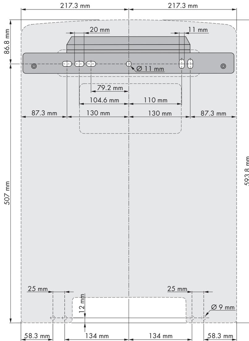
Figure 7: Position of the anchoring points
