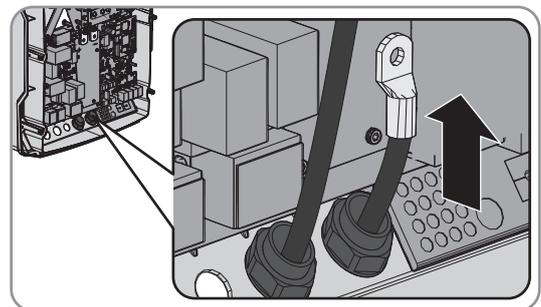
11. Route the **DC-** cable on the side of the protective cover marked with a - symbol.
