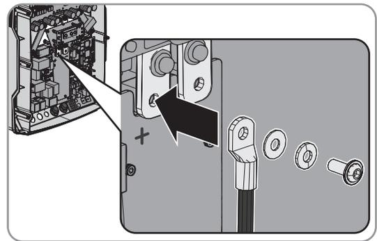
8. Ensure that the entire contact surface of the fender washer is in contact with the terminal lug.
