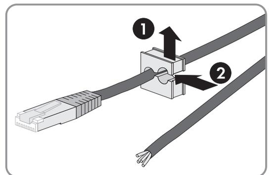
7. Open the cable feed-through plate and insert the cable support sleeves into the cable feed-through plate. Position the flat sides of each cable support sleeve on the flat side in the cable feed-through plate.
