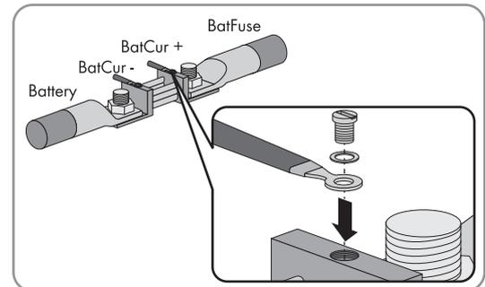
3. Close the BatFuse load-break switch quickly and switch on the Sunny Island.
