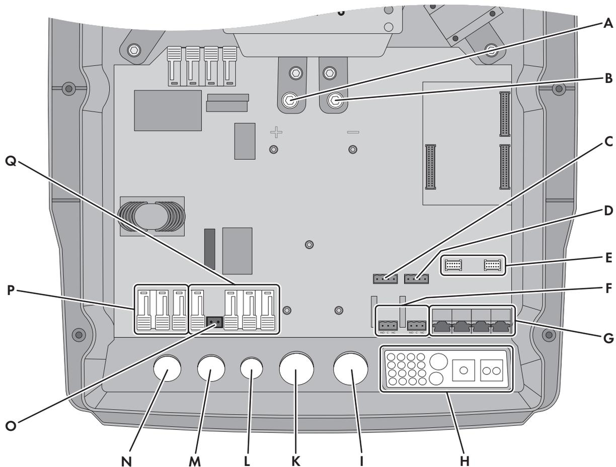
Figure 9: Connection area of the Sunny Island inverter
