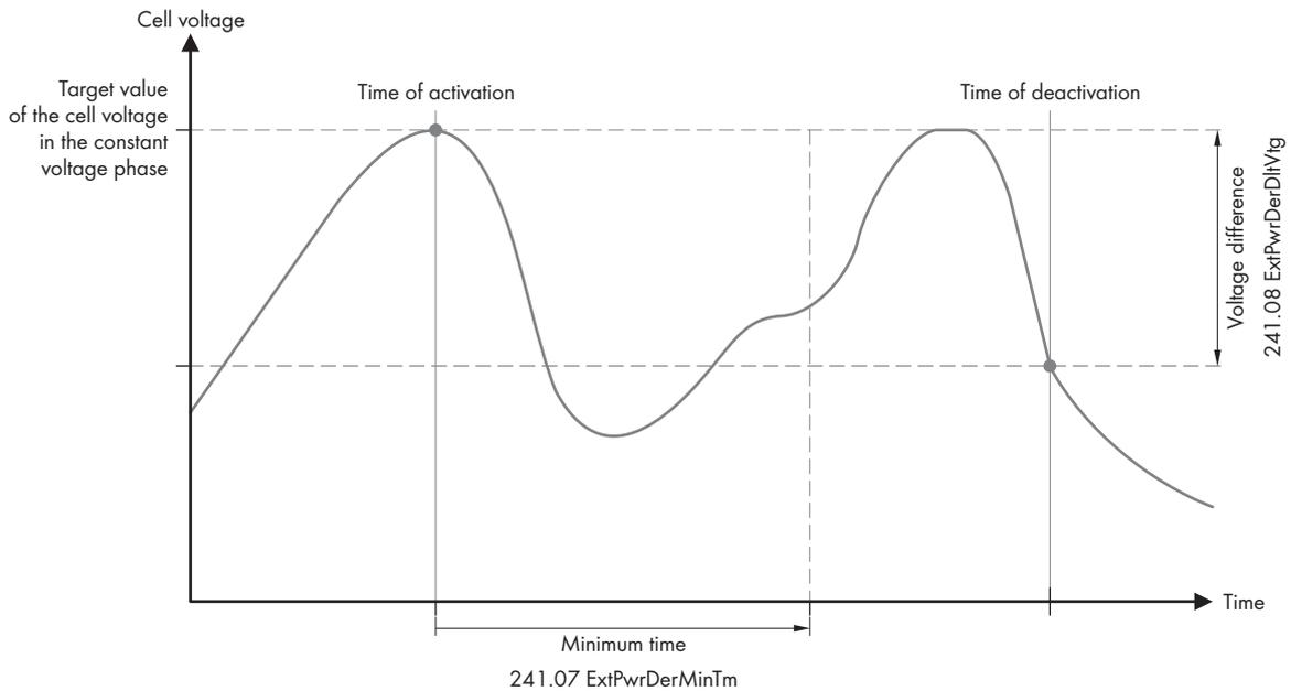
Figure 25: Switching-on time and switching-off time for utilization of excess energy during constant voltage phase
