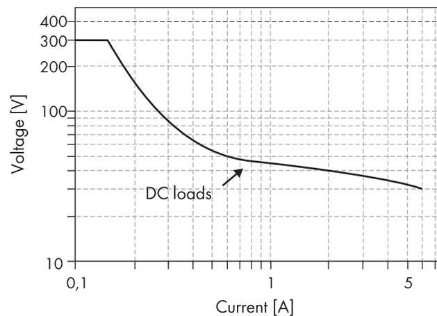
Figure 32: DC load limitation curve of multifunction relays 1 and 2
