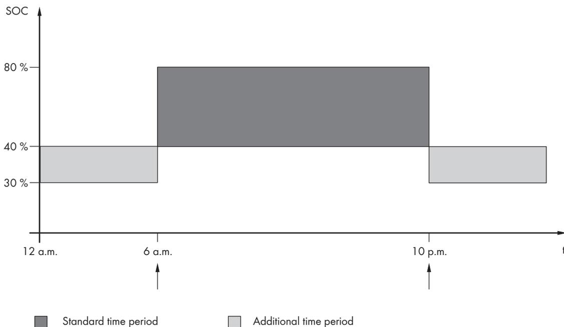
Figure 24: Profile of the SOC thresholds for controlling the load-shedding contactor and the start times for the intervals
