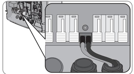
2. At the master, connect the tie switch monitoring. Ensure that the cable from **X5 3** and **X5 4** is correctly connected (see Section 7.5.6 "Connecting BatVtgOut, DigIn, BatTMP and BatCur", page 63).
