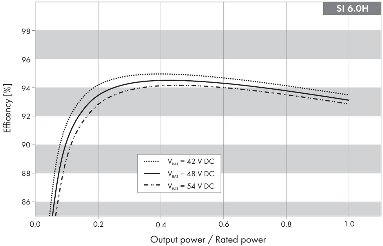
Figure 30: Characteristic efficiency curve
