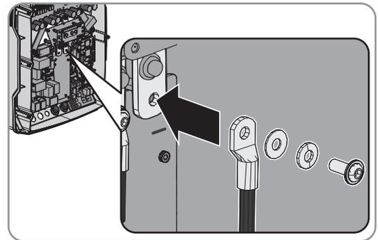
13. Ensure that the entire contact surface of the fender washer is in contact with the terminal lug.
