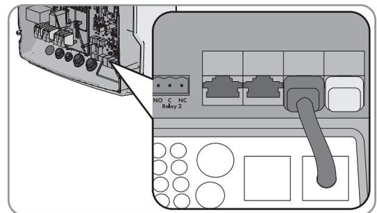
2. Connect the other end of the data cable to the battery management of the lithium-ion battery (see battery manufacturer documentation).
