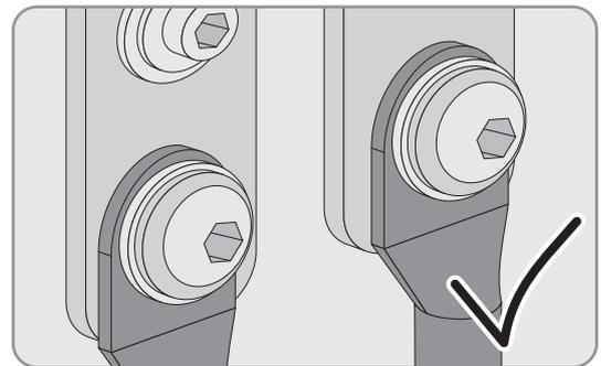
14. Tighten the swivel nuts of the cable glands (torque 4.5 Nm).
