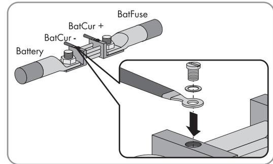
4. On the Sunny Island, connect the insulated conductors to the terminals **BatCur +** and **BatCur-**. Ensure that the cable is correctly connected (see Section 7.5.6 "Connecting BatVtgOut, DigIn, BatTMP and BatCur", page 63).
