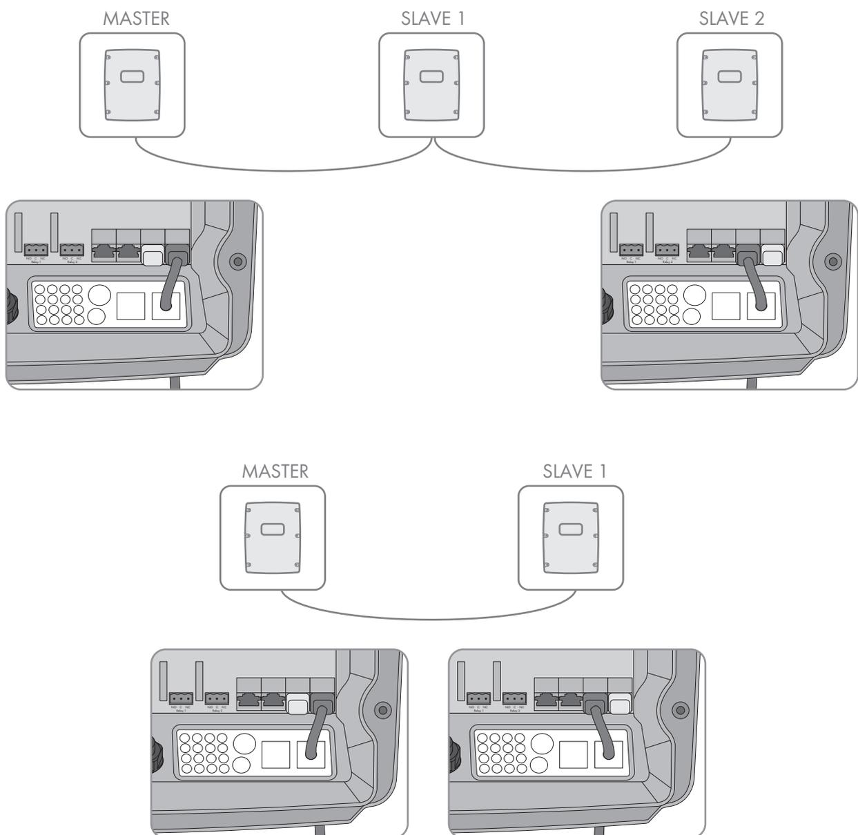
Figure 11: Internal communication cabling
