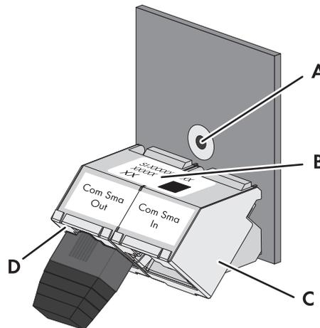
Figure 13: Design of the SI-COMSMA.BGx
