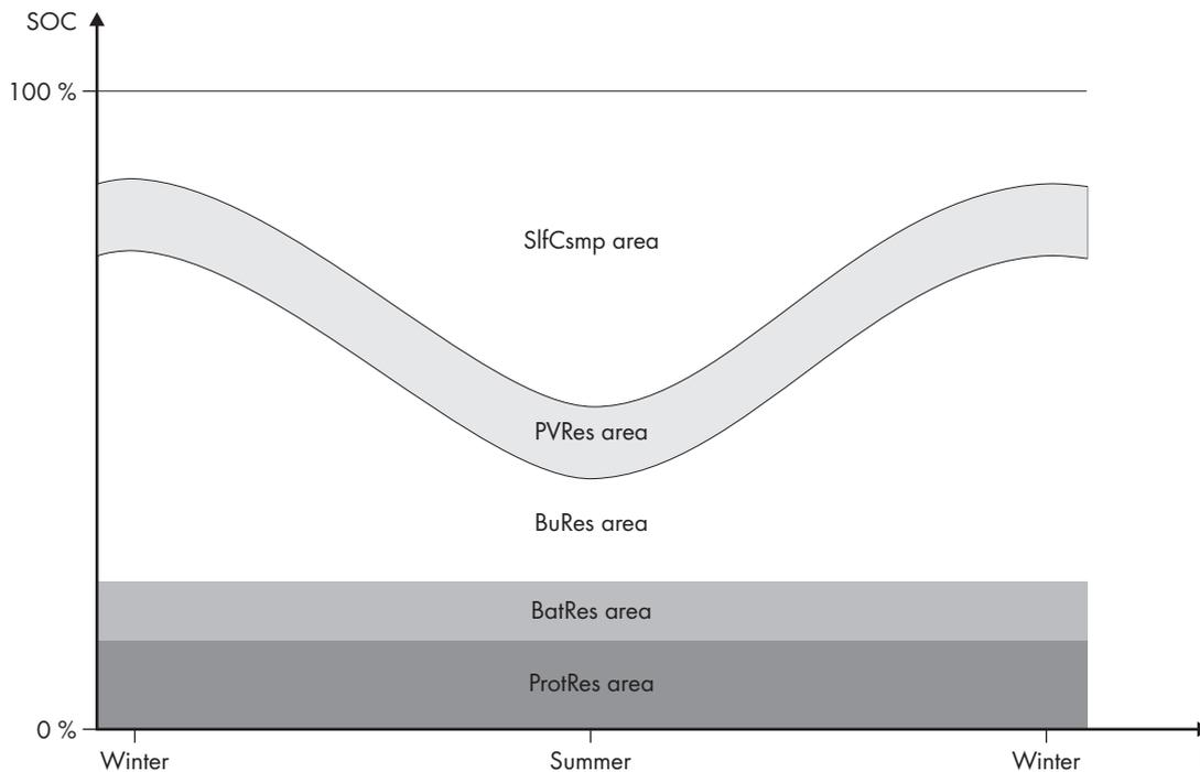
Figure 22: State of charge ranges of the battery according to the time of year (example)
