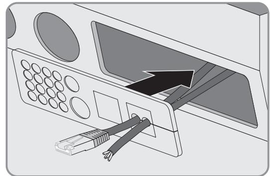
9. Hook the cable feed-through plate into the enclosure opening of the cable feed-through plate and press into the enclosure opening.
