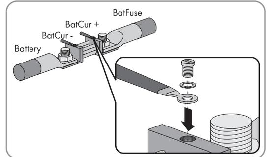
12. Connect the **BatCur-** insulated measuring conductor on the side for connecting the battery.
