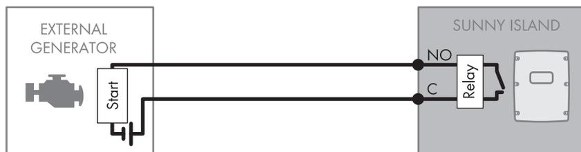
Figure 15: Connecting the Generator Control to Sunny Island
