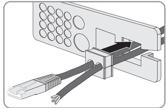
8. Hold the cables and push the cable feed-through plate to the enclosure opening of the cable feed-through plate.
