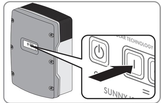
4. Switch to installer mode on the Sunny Remote Control (see Sunny Island operating manual).
