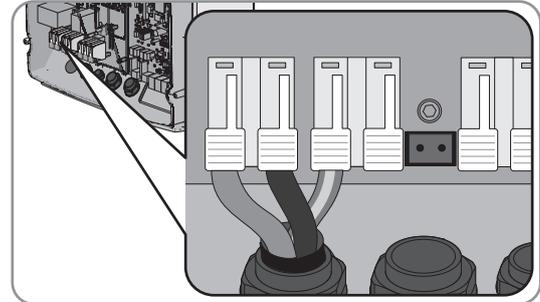
2. If the conductor cross-section of the grounding conductor is less than 10 mm<sup>2</sup>, make sure that an additional grounding conductor is connected to terminal **AC1 Loads/SunnyBoys PE** (see Section 7.5.3 "Connecting the Grounding Conductor", page 60).
