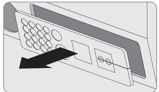
2. Retain the cable feed-through plate for later use.
