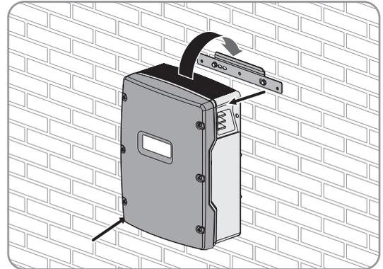
7. Mount the Sunny Island SI6.0H-11 and SI8.0H-11 to the wall mounting bracket. For this, use the side recess grips or a steel rod (diameter: maximum 30 mm). Keep the Sunny Island in a horizontal position when moving it.
