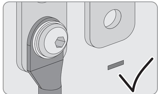
9. Strip off the insulation of the **DC-** cable and mount a terminal lug.
