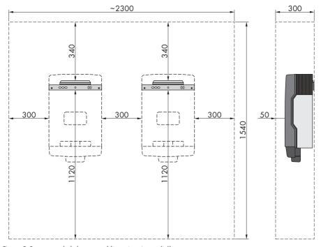
Figure 5: Recommended clearances (dimensions in mm (in))
