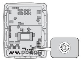
Figure 12: Positions of rotary switch C
