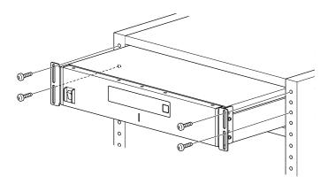
Screws used for attaching to a rack are not included in the set. Please use screws attached with a rack.
