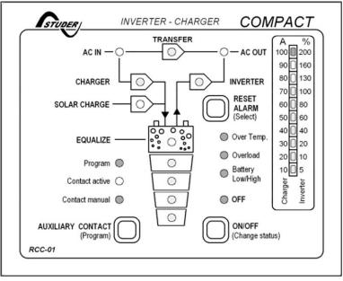
The output power and the charging currents are displayed on the remote control. In the remote control there is an additional alarm contact and a built-in control Input. These two functions are available through Tip-jack RJ11/4 for use. This auxiliary contact is Front / Work contact (max. 0.5A!), which is independent from the auxiliary
