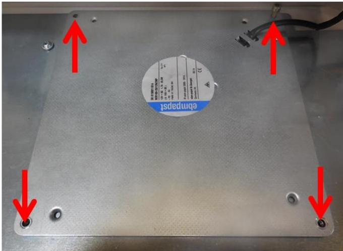
Figure 32: Removing the fan
