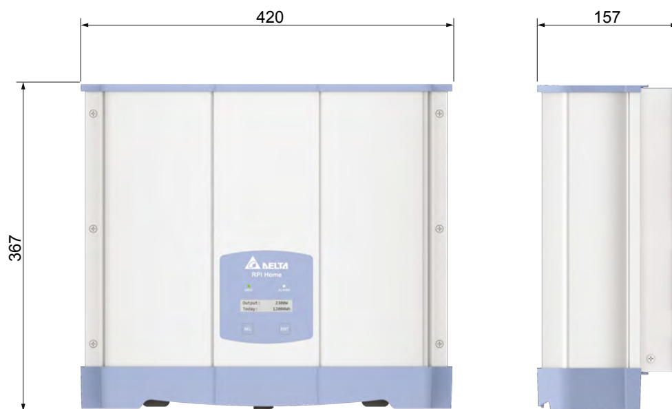
Fig. 5.6: Dimensions of the inverter in mm
