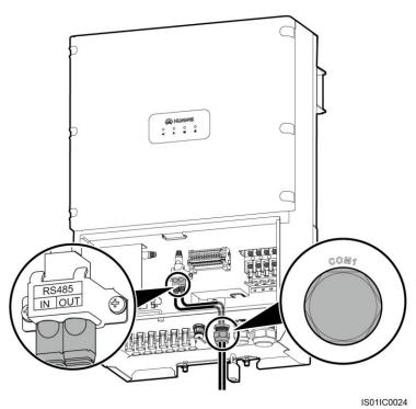
Figure 5-28 Connecting RS485 communications cables
