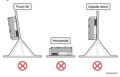
Figure 4-23 Incorrect installation modes
