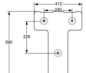
Figure 2-9 Rear panel dimensions (unit: mm)
