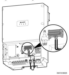
e. Bind the communications cables after connecting them, as shown in Figure 5-26.
