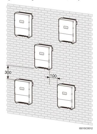
Figure 4-8 Triangle installation mode (if the space is insufficient, unit: mm)
