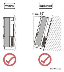
• Do not install the SUN2000 at a front tilt, excessive back tilt, or side tilt, horizontally, or upside down.
