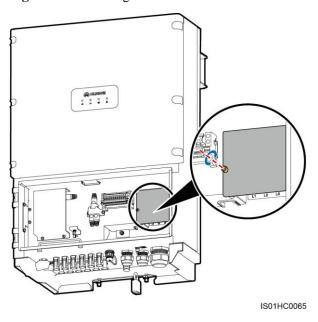
**Step 2** Remove the support bar, as shown in Figure 5-31.
