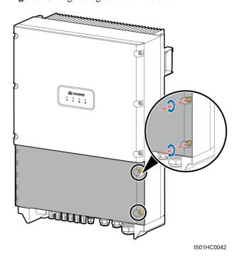
Figure 5-32 Tightening screws on the door
