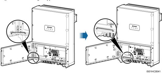
**Step 3** Close the chassis door and tighten the two screws on the door to a torque of 4 N m, as shown in Figure 5-32.
