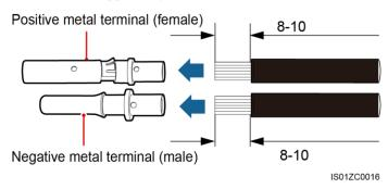
**Step 2** Insert the exposed area of the positive and negative power cables into the metal terminals of the positive and negative connectors respectively and crimp them using a crimping tool, as shown in Figure 5-15. Ensure that the cables are crimped tightly such that they cannot be pulled out by a force less than 400 N.
