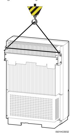
**Step 6** Mount the SUN2000 on the rear panel and keep them aligned with each other, as shown in Figure 4-18.
