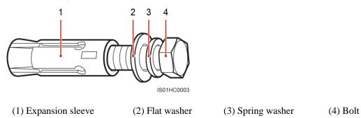
**Figure 4-13** Drilling a hole and installing an expansion bolt (unit: mm)
