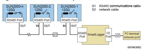
Figure 5-21 Communication mode for multiple SUN2000s
