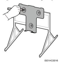
**Step 2** Drill holes using a hammer drill, as shown in Figure 4-27.
