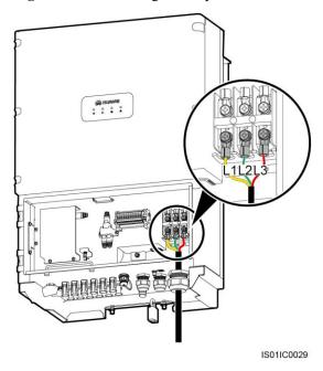
Figure 5-10 Connecting AC output cables for the SUN2000-40KTL
