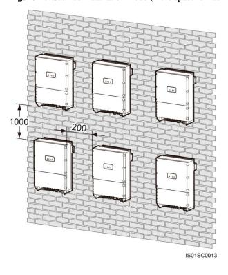
Figure 4-9 Stacked installation mode (if the space is insufficient, unit: mm)
