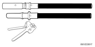
**Step 3** Insert the crimped positive and negative power cables into the corresponding positive and negative connectors until a "click" sound is heard.
