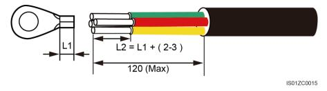
Figure 5-8 Stripped length for the SUN2000-40KTL (unit: mm)
