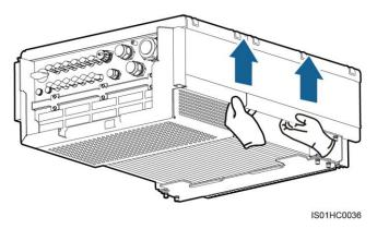
**Step 2** Carry the SUN2000 out of the packing case and move it to the installation position.
