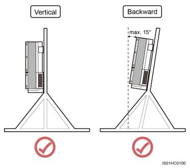
• Do not install the SUN2000 at an excessive front or back tilt, at a side tilt, horizontally, or upside down.
