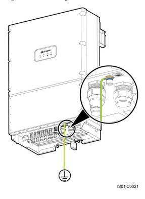
Figure 5-3 Connecting the PGND cable
