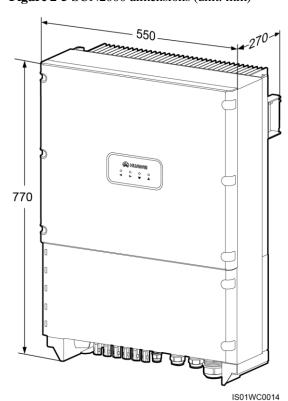
Figure 2-5 SUN2000 dimensions (unit: mm)
