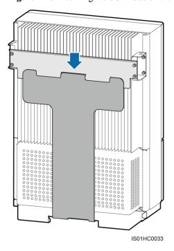
Figure 4-18 Mounting the SUN2000 on the rear panel
