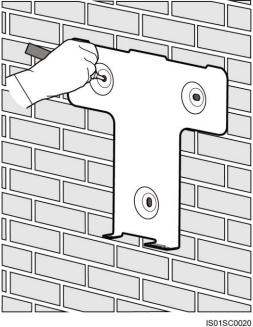
**Step 2** Drill holes using a hammer drill and install expansion bolts, as shown in Figure 4-13.
