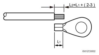
**Step 2** Insert the exposed core wires into the crimping area of the OT terminal and crimp them using hydraulic pliers, as shown in Figure 5-2.
