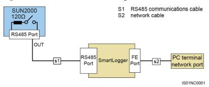
• Figure 5-21 shows the communication mode for multiple SUN2000-33KTL/40KTLs. If multiple SUN2000-33KTL/40KTLs are used, connect all the SUN2000s in daisy chain mode over an RS485 communications cable.
