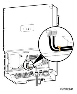
Figure 5-29 Binding communications cables
