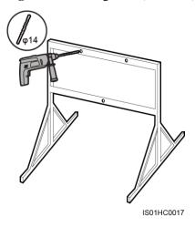
**Step 3** Align the rear panel with the hole positions, insert M12x40 bolts (expansion bolts without expansion sleeves) into the holes through the rear panel, secure them using the shipped stainless steel nuts and flat washers, and tighten the bolts to a torque of 45 N m using a torque wrench, as shown in Figure 4-28.
