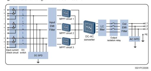
Figure 2-13 Circuit diagram for the SUN2000-40KTL
