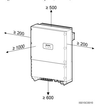
Figure 4-6 Installation space (unit: mm)
