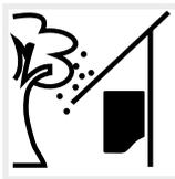
Protect inverter from falling parts which could enter the inverter's ventilation openings.
