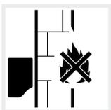
Mount inverter on a non-flammable installation surface.
