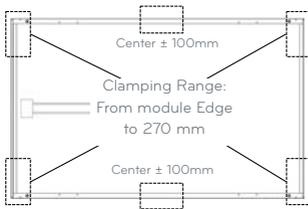
Use four clamps on the short frame and two clamps at the center of the long frame.
