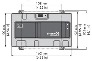
Figure 4: Dimensions for wall mounting
