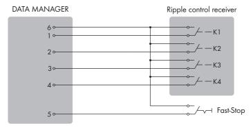
Figure 7: Connection of a Ripple Control Receiver
