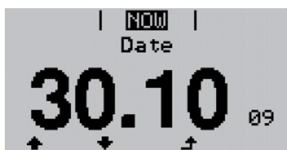
Date If the date is changed on an inverter or a system add-on, it will also be changed in any other devices that are connected via Fronius Solar Net.
